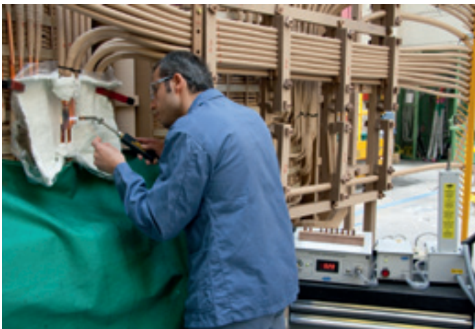
∨ Brazing of a 40 MVA 230 kV winding lead
