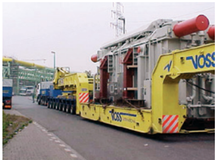
Special transport of a generator step-up transformer for the German utility RWE - 332 MVA water cooled; 115/21 kV
