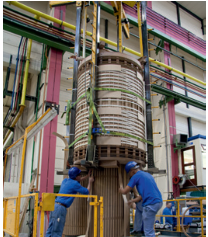
Coil assembly of a 60MVA 230/27.5/27.5 kV trackside transformer >
